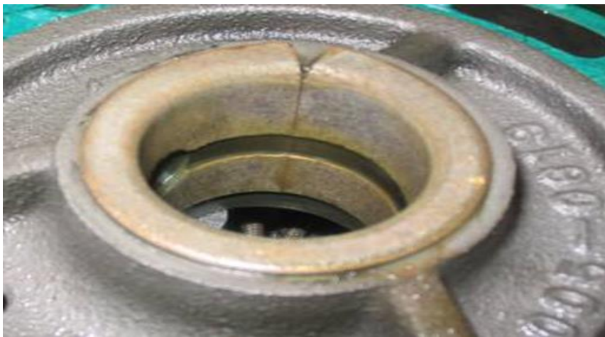
Rebuilder 3DS-1000-TSE Worn Housing cover Bearing
